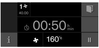
The appliance goes into standby mode. The display shows the operating mode, the temperature, the cooking time and the remaining time until the start. The appliance starts at the calculated time and automatically switches off once the cooking time has elapsed.
