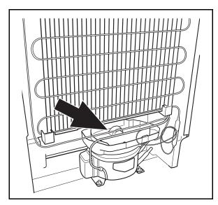
To prevent the evaporation pan from overflowing in this case, mop up the condensation with a sponge.
