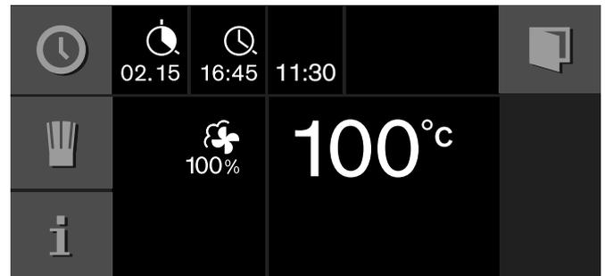
The appliance switches to standby. The heating mode, temperature, cooking time and cooking time end appear in the display. The appliance starts at the calculated time and switches off automatically when the cooking time has elapsed.
