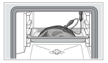
If there are several pieces of food, stick the core temperature probe into the middle of the thickest piece.
