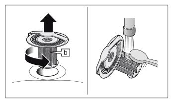
10 Insert the drain filter and turn right to the stop.Press ✓ to confirm.
