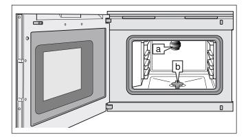
The cleaning program removes stubborn dirt. A cleaning cartridge (a) is screwed into the top of the cooking compartment. The cooking compartment is cleaned, rinsed, and dried completely automatically. The drain filter (b) must remain inserted in the cooking compartment floor while the cleaning program is in progress.
