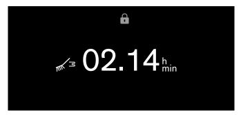
After the descaling program has finished, a signal sounds. The appliance door is unlocked. A message appears on the display.
