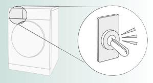
The automatic cleaning process causes a clicking noise.
