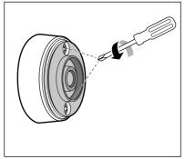
2 Remove the upper section of the casing. Remove the old battery. Insert the new battery. Make sure that the polarity is correct.
