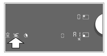
Within the next 10 seconds, select the required temperature setting using the twist knob.
