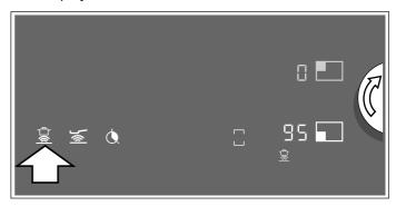
6 Set the required temperature using the twist knob. The temperature can be changed by increments of 5 °C.
