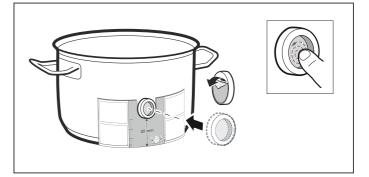
Press the silicone patch down, and press on its inside surface too.
