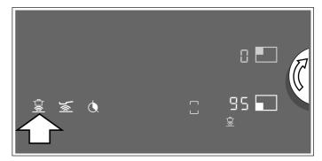
6 Set the required temperature using the twist knob. The temperature can be changed by increments of 5 °C. 7 The hotplate display shows the progress of the heating process from \_ to \_ and flashes alternately with the set temperature. Once the set temperature has been reached, an audible signal sounds and the heating indicator goes out. The selected temperature will then be displayed again.
