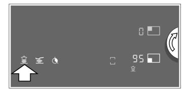
Set the required temperature using the twist knob. The temperature can be changed by increments of 5 °C. 7 The hotplate display shows the progress of the heating process from \_ to \_ and flashes alternately with the set temperature. Once the set temperature has been reached, an audible signal sounds and the heating indicator goes out. The selected temperature will then be displayed again.
