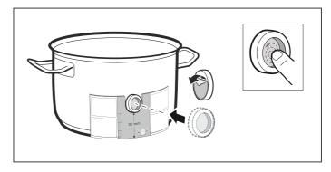
Press the silicone patch down, and press on its inside surface too.
