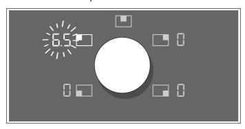
2 Set the cookware down on a flexible hotplate within the next 90 seconds. The new hotplate is detected and the 🗇 symbol lights up. The heat setting that has been applied flashes in the hotplate display.
