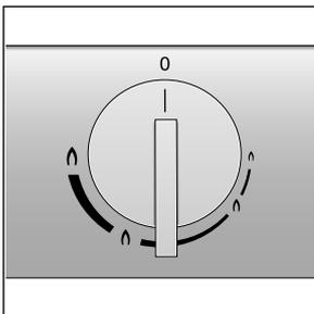
The markings show the setting between high and low heat. The flame setting is infinitely variable between high and low.
