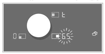
3 Select the new hotplate within 90 seconds using the twist knob. The setting has been transferred.
