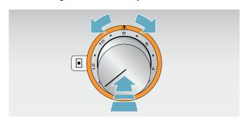
Turn the control knob to set the heat setting.
