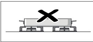
Do not heat a cooking vessel (e.g. roaster, pan, grill stone) on more than one burner at the same time. The resulting heat accumulation will damage the appliance.
