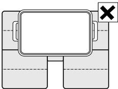
The vessel must not cover the two side cooking zones and the FlexPlus cooking zone at the same time.
