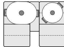
To link the FlexPlus cooking zone to the corresponding hotplate, lift up the cookware, select a heat setting and then place the cookware back down.
