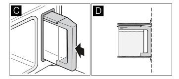
The tank must be flush with the tank slot (Figure D).
