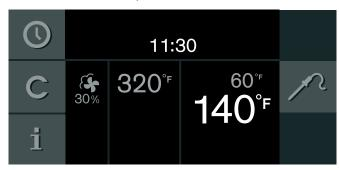
The appliance heats with the set heating function. The current core temperature is displayed and, under it, the set core temperature.
