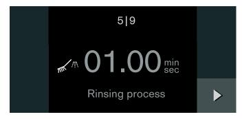
9 A signal sounds after 1 minute. Empty the evaporator tray with the cleaning sponge. Confirm with . The second rinsing operation appears. Start with ▶.
