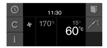
The appliance heats with the set heating mode. The current core temperature is displayed and, under it, the set core temperature. You can change the set core temperatur at any time.
