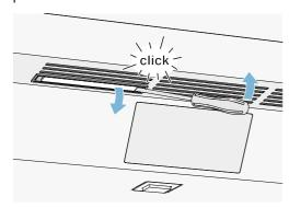
2 Remove the used odour filter and replace with a new odour filter.
