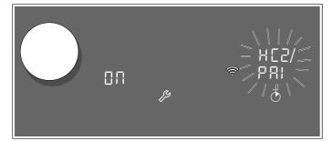
The appliance will automatically try to connect to the app.  $H \sqsubseteq 2$  and  $P R \downarrow$  will flash alternately in the settings area. The value  $\square \Pi$  will flash on the hotplate display.
