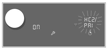
The appliance will automatically try to connect to the app.  $H \square 2$  and  $\square R \square$  will flash alternately in the settings area. The value  $\square \square$  will flash on the hotplate display.
