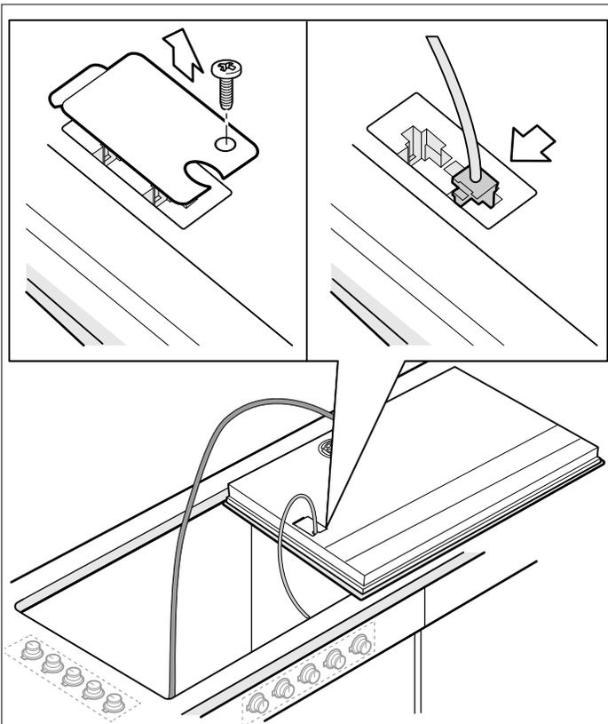
2. Evenly insert appliance into cut-out. Press appliance firmly into the cut-out.
