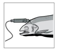
**Turning the food:** If you want to turn the food, do not remove the core temperature probe. Once you have turned the food, check that the core temperature probe is correctly positioned in the food.
