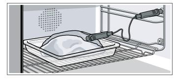
**Poultry:** Insert the core temperature probe as far as it will go into the thickest point in the breast. Depending on its structure, insert the core temperature probe into the poultry crossways or lengthways. With poultry, make sure that the tip of the core temperature probe does not protrude into the cavity in the middle of the bird.
