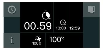
The appliance switches off after the cooking time has elapsed. The ♠ symbol flashes and a signal sounds. The signal stops when you touch the ✔ symbol, open the appliance door, or switch the function selector to 0.
