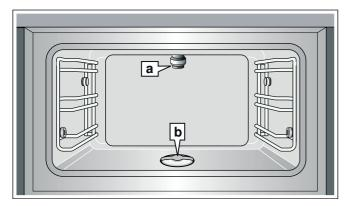
The cleaning programme removes stubborn dirt. A cleaning cartridge (a) is screwed into the top of the cooking compartment. The cooking compartment is cleaned, rinsed and dried fully automatically. The strainer filter (b) must remain inserted in the cooking compartment floor while the cleaning programme is in progress.
