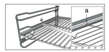
When inserting the cooking container, ensure that the lug (a) is facing upwards.
