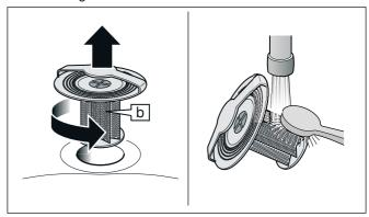
10 Insert the strainer filter and turn it clockwise as far as it will go. Press ✓ to confirm.
