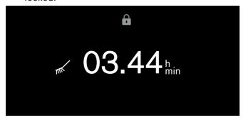
Once the cleaning programme has finished, an audible signal sounds. The appliance door is unlocked. A message appears in the display.
