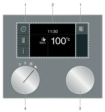
Operating controls on the lower side of the appliance
