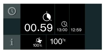
Once the cooking time has elapsed, the appliance switches off. The () symbol flashes and an audible signal sounds. The signal stops early if you touch the symbol, open the appliance door, or set the function selector to 0.
