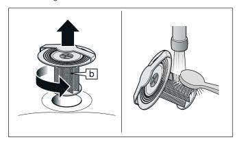
10 Insert the strainer filter and turn it clockwise as far as it will go. Press v to confirm.
