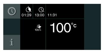
One minute before the end of the cooking time, the elapsed cooking time is shown enlarged on the display.
