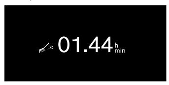
Note: After approximately 1:30 hours, a message appears in the display. Remove and drain the tank. Clean the tank thoroughly. Fill the tank with fresh water. Slide the tank into the appliance. Confirm by pressing ✓. Press ▶ to start the rinsing process.
