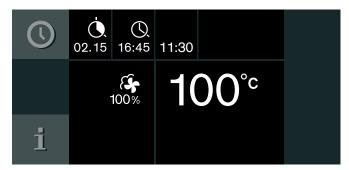
The appliance switches to standby. The display shows the operating mode, temperature, cooking time and cooking time end. The appliance starts at the calculated time and automatically switches off once the cooking time has elapsed.
