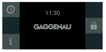
The child lock is activated. The standby screen appears. The  $\bigcirc$  symbol is shown at the top of the display.
