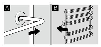
The rails fit both the left and right sides. Ensure that, as shown in figure B, the recess is below.
