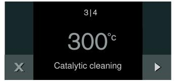
A signal sounds after the catalytic cleaning has expired. A message appears in the display. Leave the appliance to cool down.
