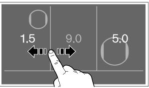
The heat setting of the combined area is the same as the heat setting of the section being expanded.
