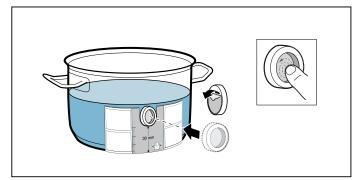
3. Press down all over the surface of the silicone patch, including in the center.
