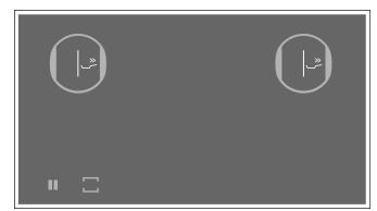
If the Pan Boost function is active and settings for a different cooking position on the same side of the cooking surface are selected, the Pan Boost function will be deactivated and heat setting 9.0 set automatically.
