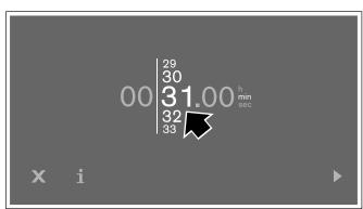
Touch the ► symbol to confirm the selected setting. The X symbol and the selected time will light up in the function bar.
