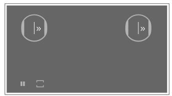
If the Power Boost function is active and you select a second cooking position on the same side of the cooking surface, the Power Boost function will be deactivated. The cooking position is automatically set to heat setting 9.0.
