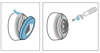
Open the cap on the cooking sensor. Remove the battery from the lower section of the casing and insert a new battery (make sure that the battery terminals (+/-) are the right way round).
