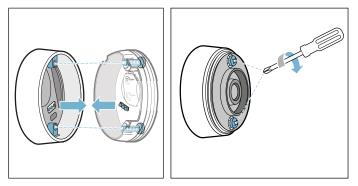
4. Put the silicone cover back on the lower section of the cooking sensor casing.
