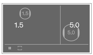
To separate the combined area again, touch one of the vertical edges of the area and swipe left or right with your finger until the hidden section reappears.
