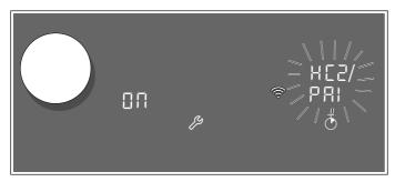
The appliance will automatically try to connect to the app.  $H \subseteq \mathcal{D}$  and  $PR \mid I$  will flash alternately in the settings area. The value  $\Pi \cap I$  will flash on the hotplate display.
