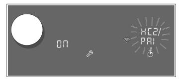
The appliance will automatically try to connect to the app.  $H \square 2$  and PR I will flash alternately in the settings area. The value  $\square n$  will flash on the hotplate display.
