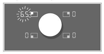
2 Set down the cookware on a flexible hotplate within the next 90 seconds. The new hotplate is detected and the symbol lights up. The heat setting that has been applied will flash in the hotplate display.
