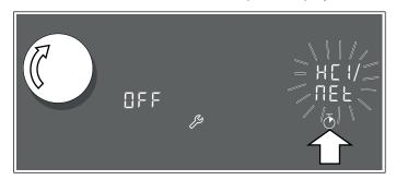
4 Set the value to  $\square \square$  using the twist knob.  $\square \square$  will flash on the hotplate display along with the symbol.
