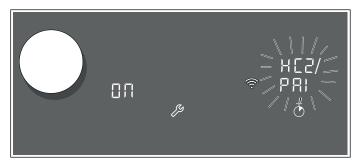
The appliance will automatically try to connect to the app.  $H \subseteq \mathcal{D}$  and  $PR \mid I$  will flash alternately in the settings area. The value  $\Pi \Pi$  will flash on the hotplate display.
