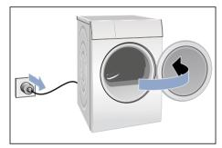
2 Remove the screws from the dryer and then remove the dryer door.
