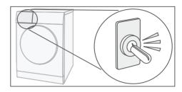
The condensation is pumped into the condensate container by a pump. This generates pumping noises.
