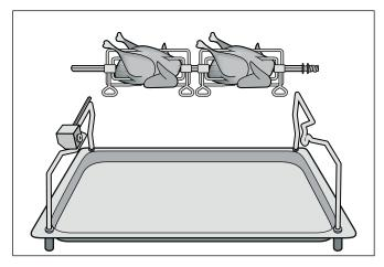
5 Set the rotary spit down onto the supporting frames. Push the rod of the rotary spit into the drive so that it engages with its square profile.
