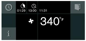
One minute before expiration of the cooking time, the expiring cooking time is enlarged in the display.
