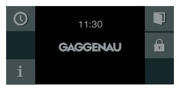
The child lock is activated. The standby screen appears. The figure at the top of the display.
