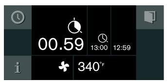
The appliance switches off after expiration of the cooking time. The nulsates and a signal sounds. It goes off prematurely if you touch the  $\checkmark$  symbol, open the appliance door or set the program selection to 0.
