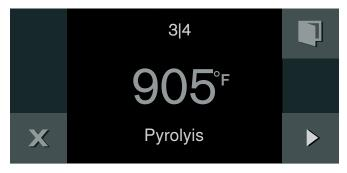
A signal sounds once the pyrolytic self-cleaning function has ended. A message appears in the display. Once the appliance has cooled down, wipe out the ash that has been left behind in the oven cavity with a damp cloth.
