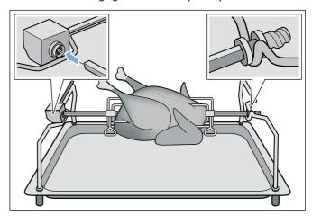
Insert the grill tray along with the rotary spit into the oven at the bottom rack level.
