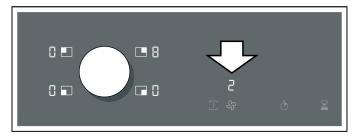
3 To set a different fan setting, touch the & symbol and use the twist knob to select the required setting.
