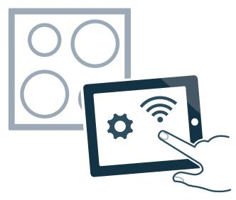
5 Use the "Home Connect" SSID and the "Home Connect" key to register your mobile device on the hob network. It can take up to 60 seconds to establish the connection.
