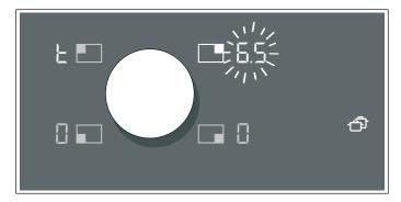
3 Use the twist knob to select the new hotplate within 90 seconds. The setting has been transferred.
