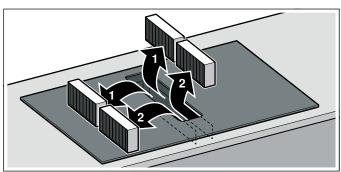
3 Insert two of the activated charcoal filters or acoustics filters into the left and right of the appliance and slide them forwards.
