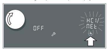
3 Set the value to ∠□∠ using the twist knob. └□∠ flashes on the hotplate display along with the symbol.
