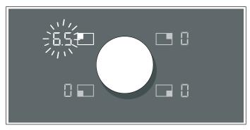
2 Set the cookware down on a flexible hotplate within the next 90 seconds. The new hotplate will be detected and the symbol will light up. The applied heat setting will flash in the hotplate display.
