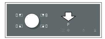
**Note:** After 6 minutes, the appliance will automatically switch back to fan setting  $\vec{J}$ .
