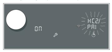
The appliance tries to connect to the app automatically.  $H \subseteq \mathcal{D}$  and PRI flash alternately in the settings area. The GR value flashes on the hotplate display.
