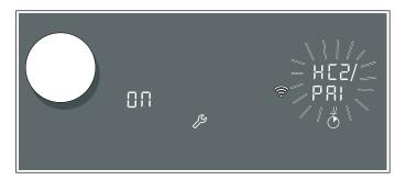
The appliance tries to connect to the app automatically. HL 2 and PR 1 flash alternately in the settings area. The  $\Pi\Pi$  value flashes on the hotplate display.
