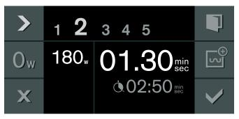
Note: You can set a stabilisation time between two microwave outputs so that the temperature is distributed evenly within the food. To do this, touch the  $O_w$  symbol and set a time using the rotary selector.
