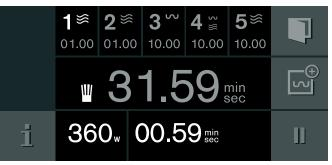
**Note:** You can use the rotary selector to change the grill setting for the full surface grill and the cooking time for a microwave output while the recipe is in progress. This does not change the saved recipe.
