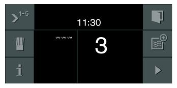
Depending on the operation mode selected, the symbol for microwave or the symbol for full surface grill appears in the right-hand control panel, which enables you to add the relevant other operation mode.
