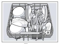
Cutlery basket a1 Large plates up to a diameter of 31 cm can be arranged in the bottom basket as shown.
