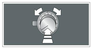
The selected heat setting will be lit on the hotplate display. The illuminated ring around the control knob will be lit.
