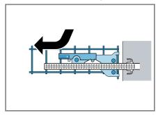
4. Slide the guide rails into the appliance.
