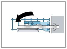
**4.** Slide the guide rails into the appliance.
