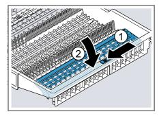
To fold down the front prongs, push the lever forwards and fold down the prongs ①.
