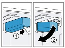
2. Turn the water filter anti-clockwise by 90° 1 and remove it 2.
