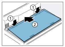
2 Grip both the front recesses at the base of the refrigerator compartment ①, lift the refrigerator compartment glass plate and remove it ②.
