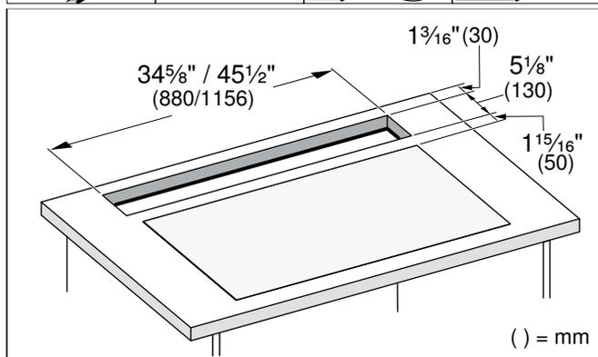
**Flush mounting:** Flush mounting into a countertop is possible.
