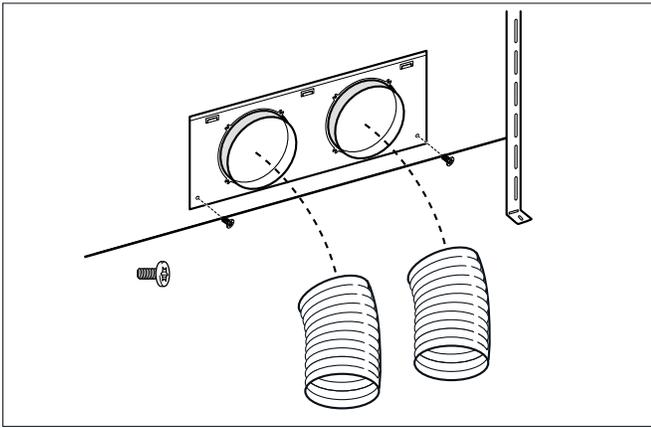
**Note:** If using an aluminum pipe, smooth the connection area beforehand.
