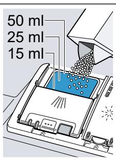
If you are using tablets, one is enough. Insert the tablets in a horizontal position.
