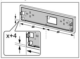
The distance between the lower edge of the retaining plate and the lower edge of the furniture panel is x + 4 mm.
