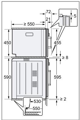
4. Observe the clearances when installing in a tall unit.
