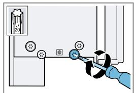
6. Slide the appliance into the built-in recess.
