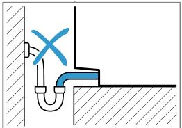
**5.** Do not place the outlet hose higher than the bottom edge of the appliance at any point.
