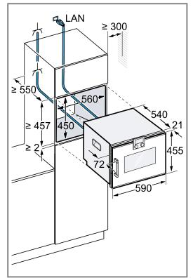
6. If there is no intermediate floor above the appliance, secure the appliance against tipping in the unit. Secure 2 commercially available brackets on both sides in the unit at a depth of 450 mm, 5 mm above the height of the appliance.
