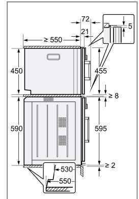
5. Observe the clearances when installing in a tall unit.
