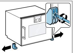
2. Remove the transport brackets for the inlet and outlet hose.
