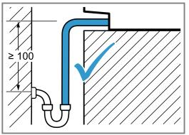
**3.** Do not place the outlet hose more than 500 mm below the drainage connection at any point.
