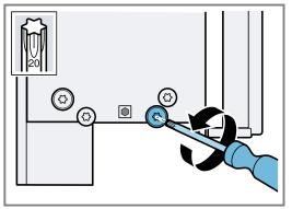
**3.** Adjust the appliance door using the grub screw. Open the appliance door and then close it again if necessary.
