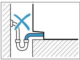
5. Do not place the outlet hose higher than the bottom edge of the appliance at any point.
