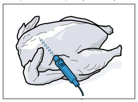
**3.** With poultry, ensure that the tip of the core temperature probe does not protrude into the cavity in the middle of the bird.
