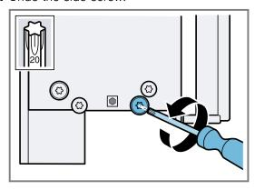
3. Adjust the appliance door using the grub screw. Open the appliance door and then close it again if necessary.
