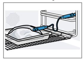
2. If there is more than one piece of meat, insert the core temperature probe into the middle of the thickest piece.
