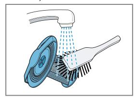
4. If it is very dirty, rinse out the drain filter under running water or clean it in the dishwasher.
