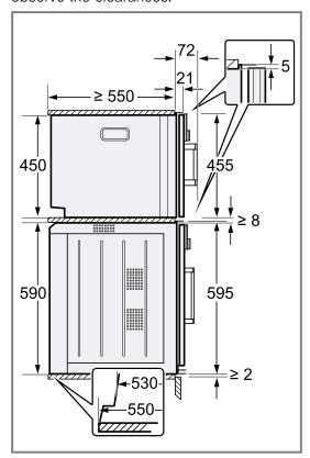
5. Observe the clearances when installing in a tall unit.
