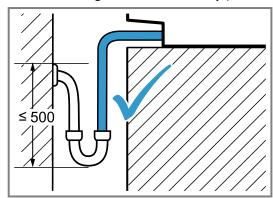
**4.** The drainage connection must not be higher than the appliance.
