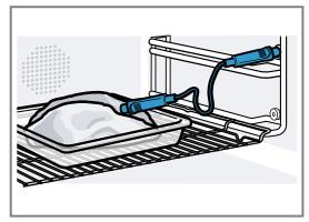
2. If there is more than one piece of meat, insert the core temperature probe into the middle of the thickest piece.
