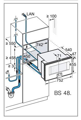
**4.** When installing 2 appliances on top of each other, observe the clearances.
