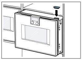
8. Slide the appliance into the built-in recess.
