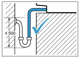
4. The drainage connection must not be higher than the appliance.
