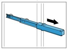
2. Move the lock in the direction of the arrow 1 and loosen the pin from the rear 2.
