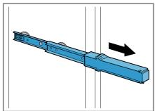
2. Move the lock in the direction of the arrow ① and loosen the pin from the rear ②.
